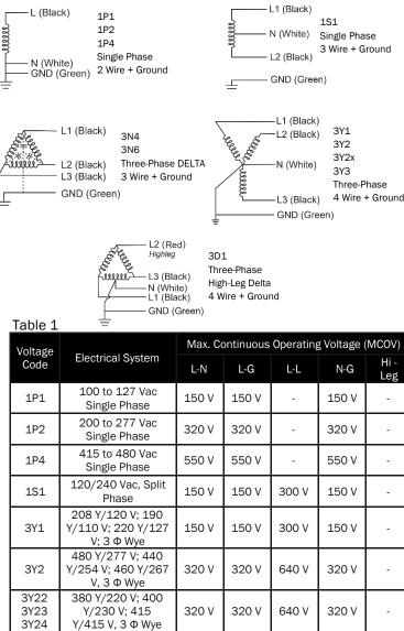
120/240 Vac, 3 Ф, 3D1 150 V 150 V 320 V 150 V 320 V High-Leg Delta 120 Vac, 3 Φ Delta 150 V 3N1X 150 V or Wye 440 to 480 Vac, 3 Φ 550 V 3N4 550 V \_ \_ Delta or Wye 525 to 600 Vac, 3 Φ 840 V 3N6 840 V Delta or Wye Installation Voltage Measurement Worksheet Measurement Measure Measure Measurement
